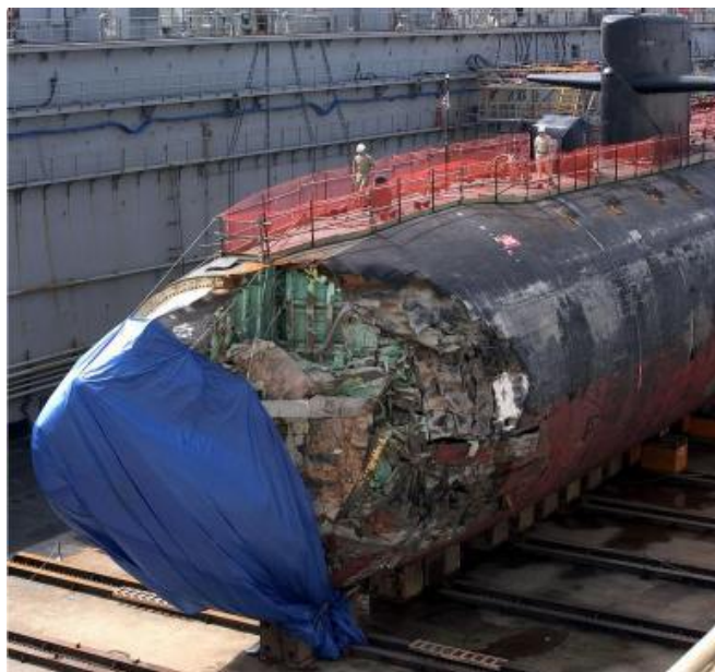
The USS San Francisco submarine ran aground on an underwater mountain that was not shown on its outdated charts
