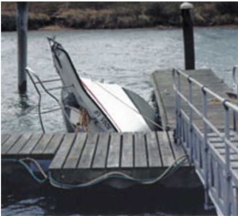
Not a scene you want to face. It doesn't take much to hold a float switch down. Switches should be oriented so that they are clear from interference and secured to the bilge floor. This boat sank when its bilge pump switch was blocked by the hose.
